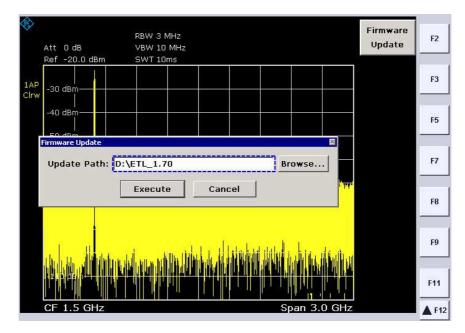
If the firmware is installed from a USB memory stick or a USB hard disk and if the update path differs from the preset path, correct the path settings by means of the **Browse** button. For this purpose, first select the drive using **Path** in the displayed dialog. Under **Files**, select the folder that contains the **ETL.package** installation files.
